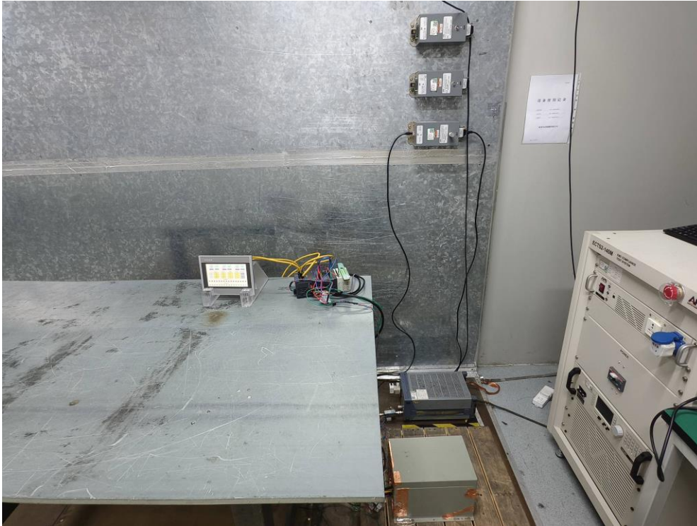
Photograph 2: Set-up for conducted emission, Ethernet ports
