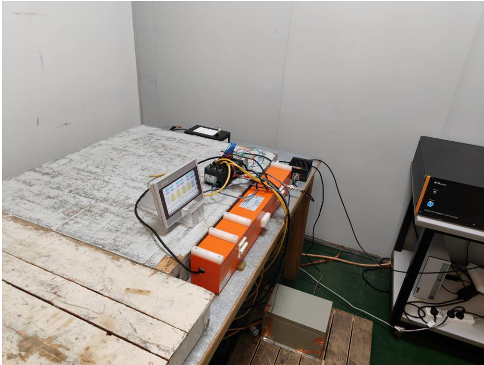
Photograph 11: Set-up for continuous induced RF disturbances, Signal Ports
