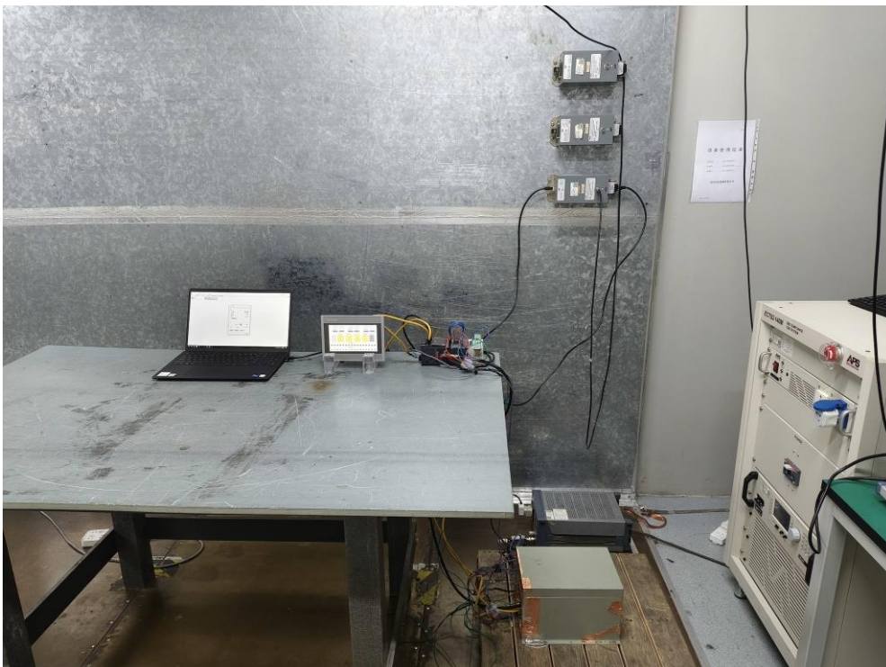
Photograph 2: Set-up for conducted emission, Ethernet ports
