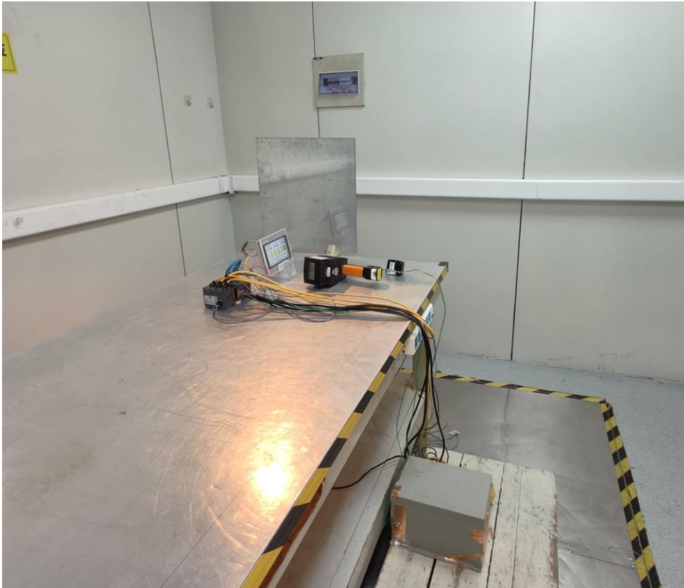
Photograph 6: Set-up for RF radiated immunity test
