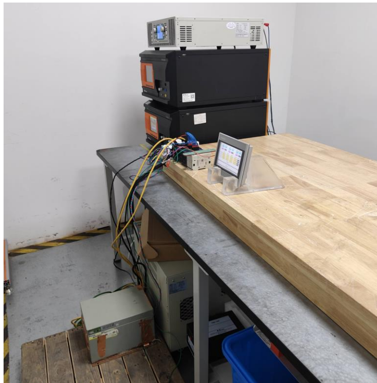
Photograph 8: Set-up for fast transients and surges, DC power port
