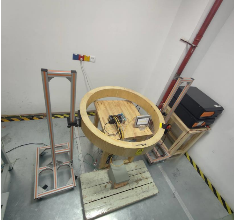
Photograph 8: Set-up for fast transients and surges, DC power port
