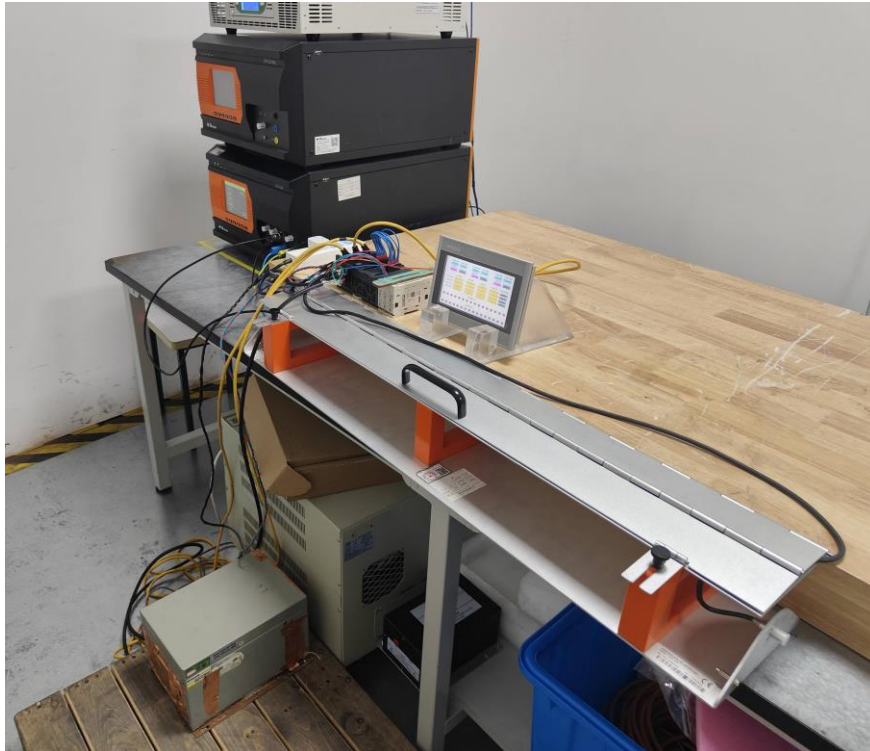
Photograph 10: Set-up for continuous induced RF disturbances, DC power port
