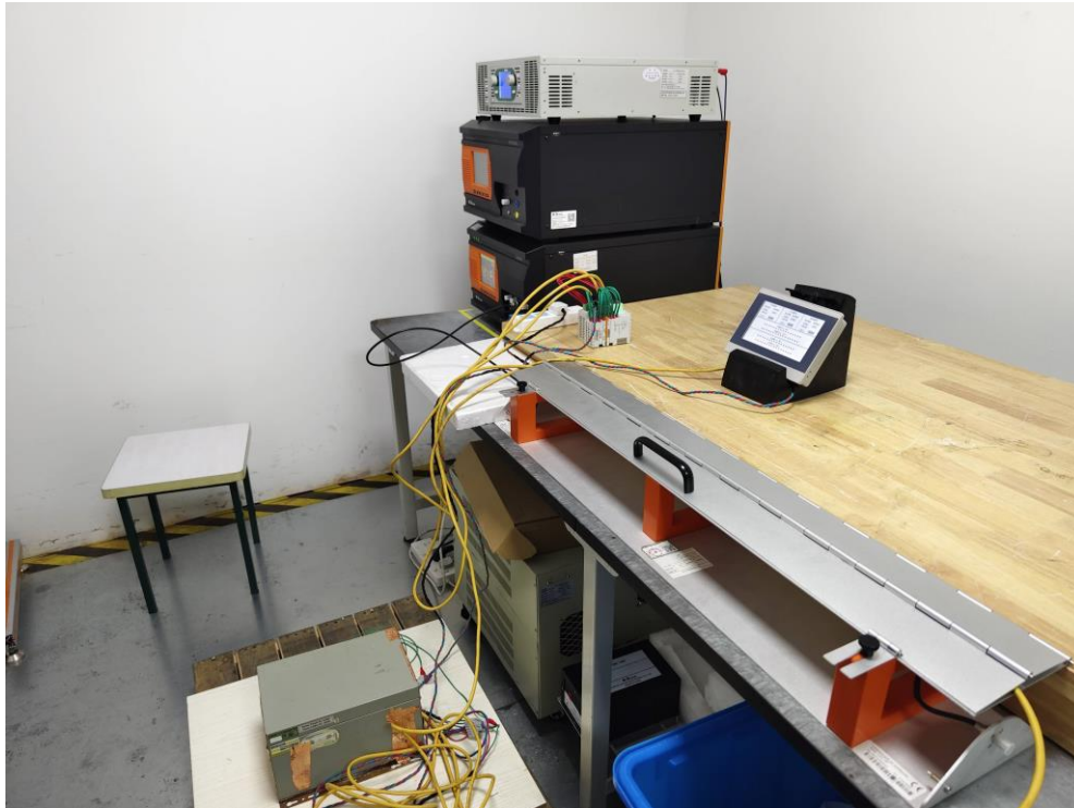
Photograph 10: Set-up for continuous induced RF disturbances, DC power port
