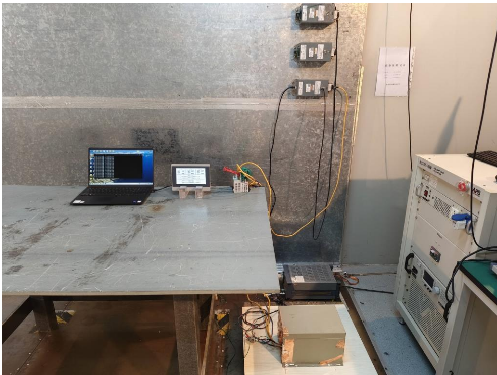
Photograph 2: Set-up for conducted emission, Ethernet ports
