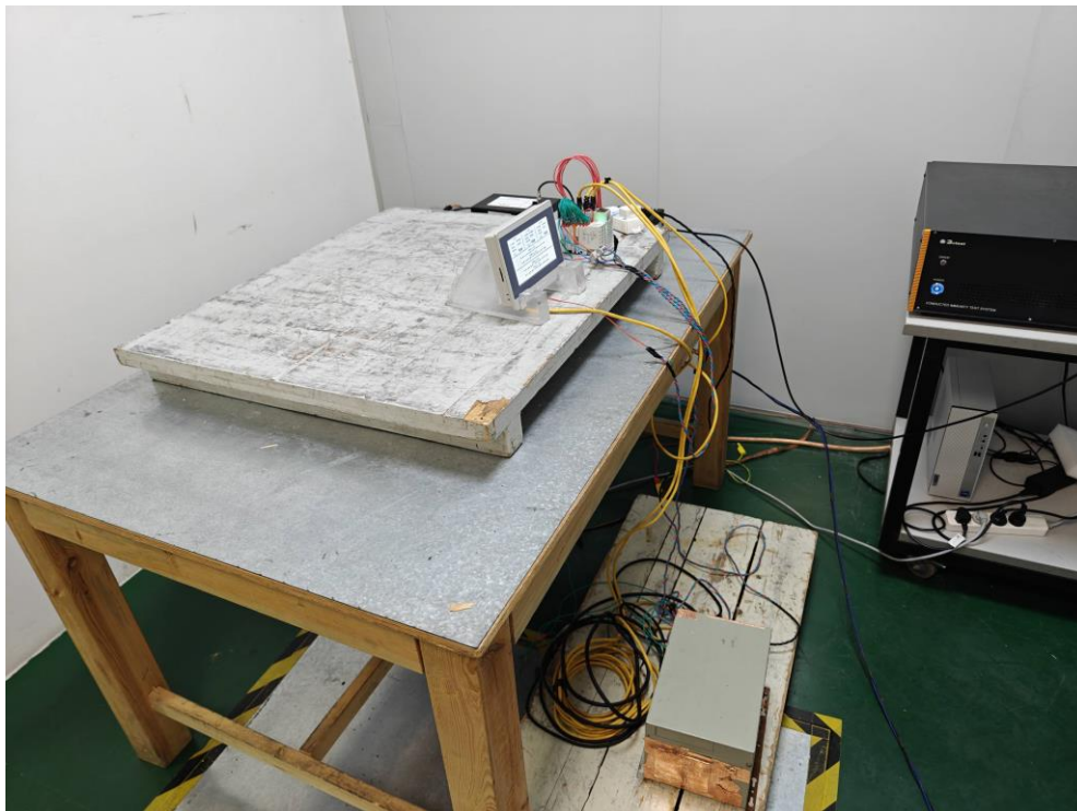
Photograph 10: Set-up for continuous induced RF disturbances, DC power port
