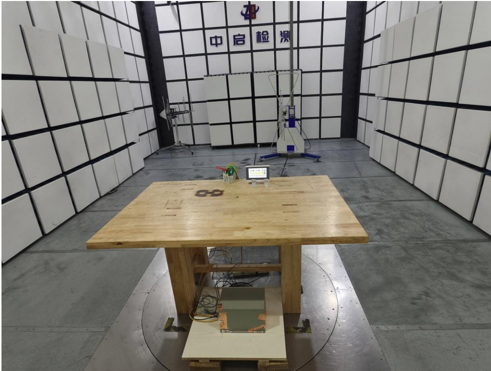
Photograph 4: Set-up for radiated emission, Above 1GHz
