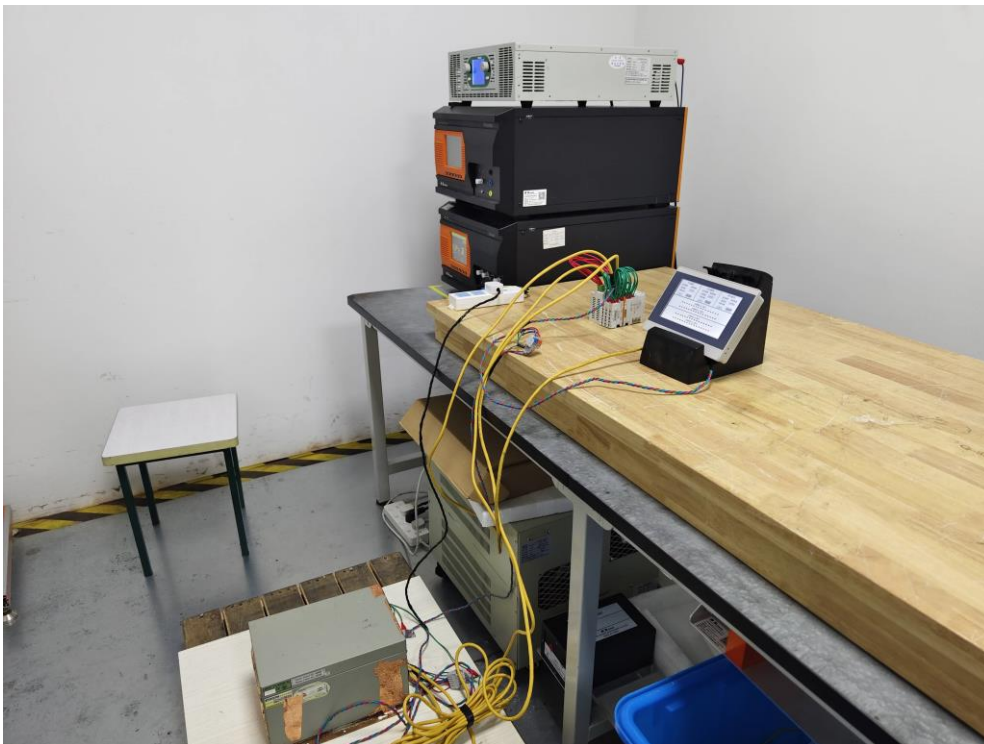
Photograph 8: Set-up for fast transients and surges, DC power port
